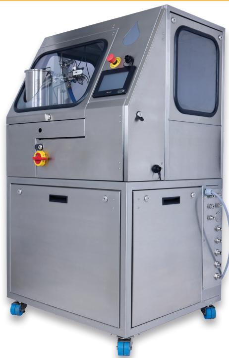
The ShearJet HP350 V2 series electric-hydraulic processor operates with a single multiplier pump which processes 100 mL sample sizes and high flow rates in distinct passes or continuous runs. This ability makes the HP350 V2 processor a viable option for R&D and pre-pilot scale applications. It is easily portable between lab suites because no utility air is required and its small foot print includes wheels.
