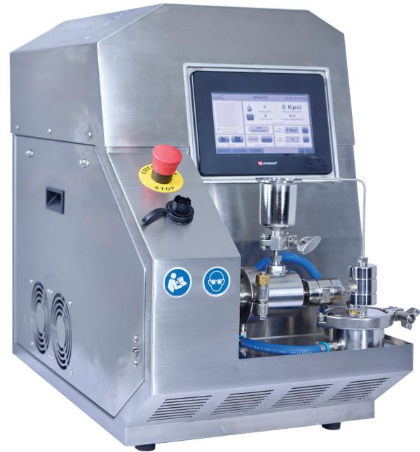
The ShearJet HL60 electric hydraulic processor is a unique R&D model designed to process samples as small as 3 mLs in distinct passes or continuous runs. Multiple samples may be processed in a short time span. Small dead volume, fewer high pressure connections and self-priming leads to reduced waste. The HMI touchscreen display puts simplicity at your fingertips, displaying relevant information in real time.
