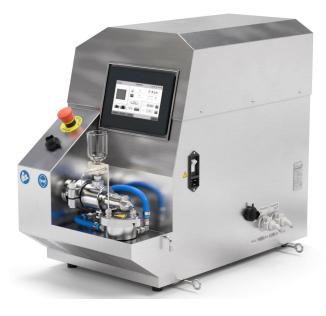
The ShearJet HL60 electric hydraulic processor is a unique R&D model designed to process samples as small as 3 mLs in distinct passes or continuous runs. Multiple samples may be processed in a short time span. Small dead volume, fewer high pressure connections and self-priming leads to reduced waste. The HMI touchscreen display puts simplicity at your fingertips, displaying relevant information in real time.
