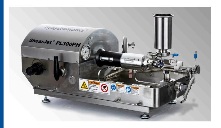
The ShearJet PL300 series processor is offered in two versions: ShearJet PL300, and ShearJet PL300PH pharma grade with USP Class VI seals, O-rings, gaskets, and electro-polish (EP) and passivation of product contact components. The ShearJet PL300 pneumatic processor runs sample sizes from 45 mLs in distinct passes or continuous runs. By decreasing high pressure piping connections, leakage possibilities are reduced as well.
