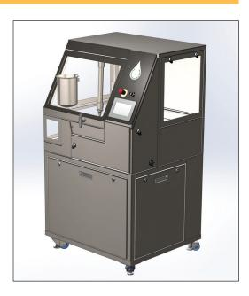
The ShearJet HP350 V2 series electric-hydraulic processor operates with a single multiplier pump which processes 80 mL sample sizes and high flow rates in distinct passes or continuous runs. This ability makes the HP350 V2 model a viable option for R&D and pre-pilot scale applications. It is easily portable between lab suites because no utility air is required and its small foot print includes wheels.
